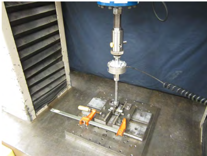
Photo No. 4 ASTM D 790 Flexural Test Setup (Ultraviolet Resistance)
