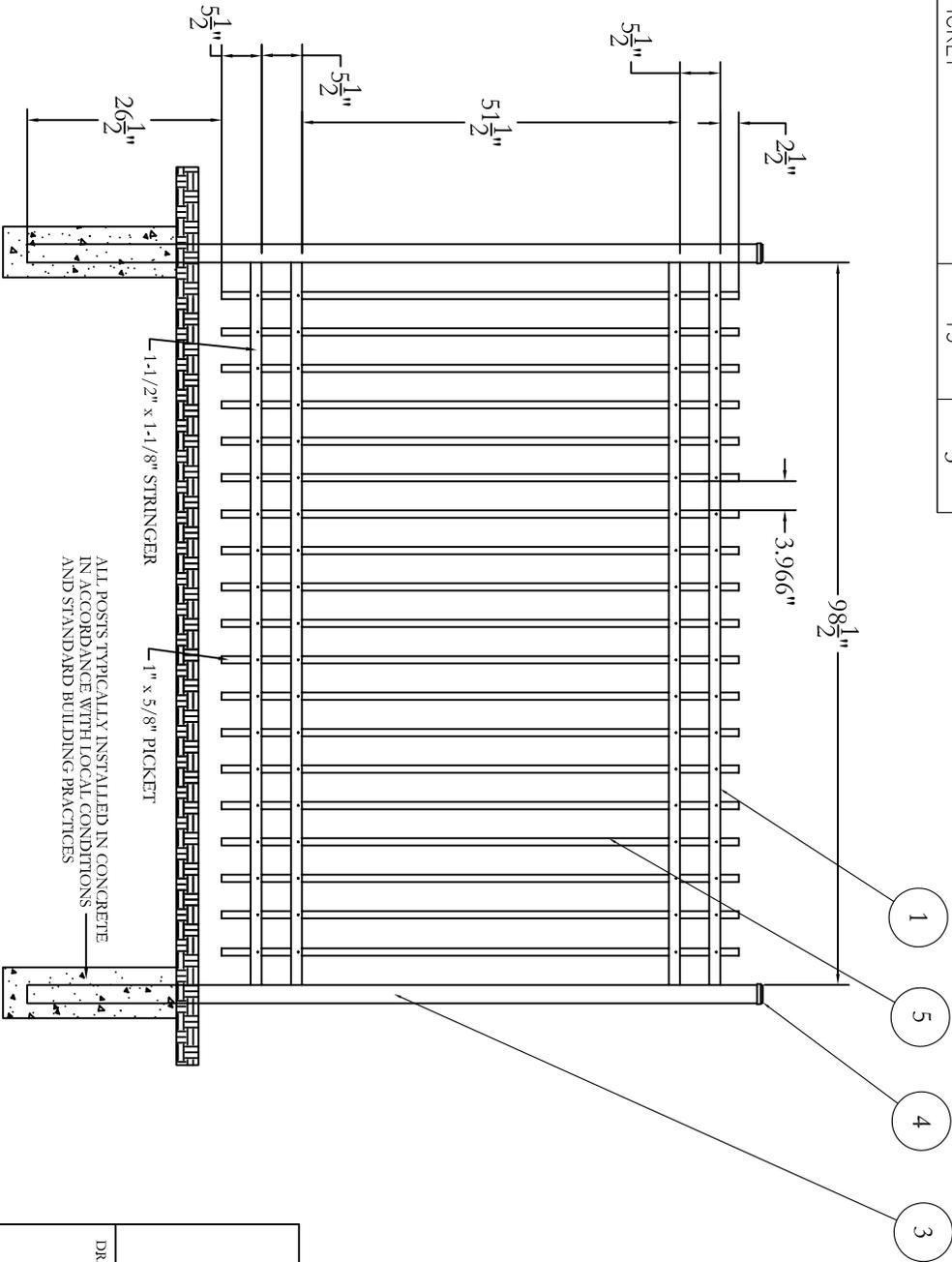
ALL POSTS TYPICALLY INSTALLED IN CONCRETE IN ACCORDANCE WITH LOCAL CONDITIONS AND STANDARD BUILDING PRACTICES
